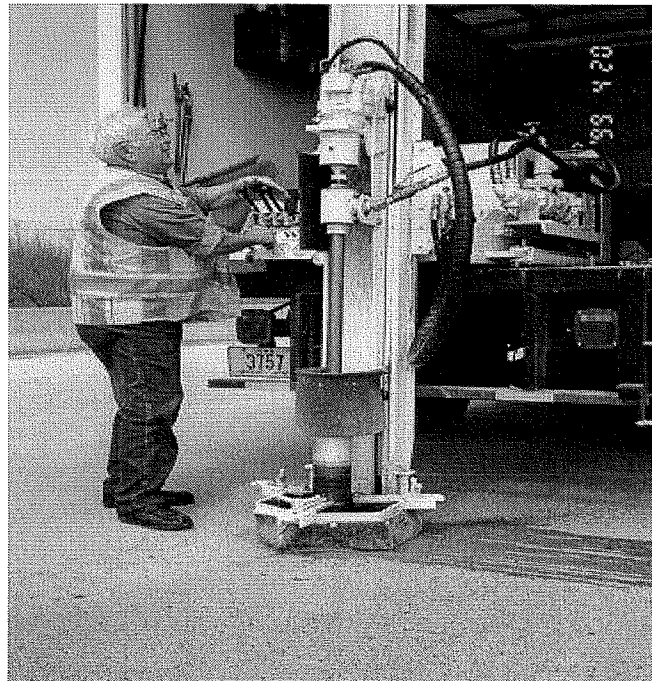
Figure 4.2 The Set Up of the Coring Process
