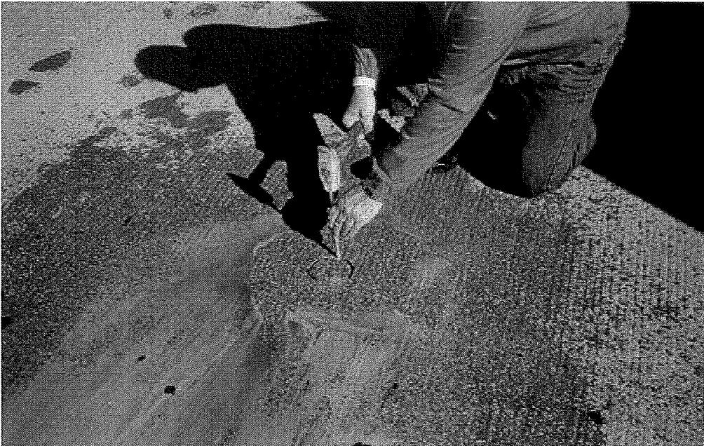
Figure 4.3 Breaking the Core
